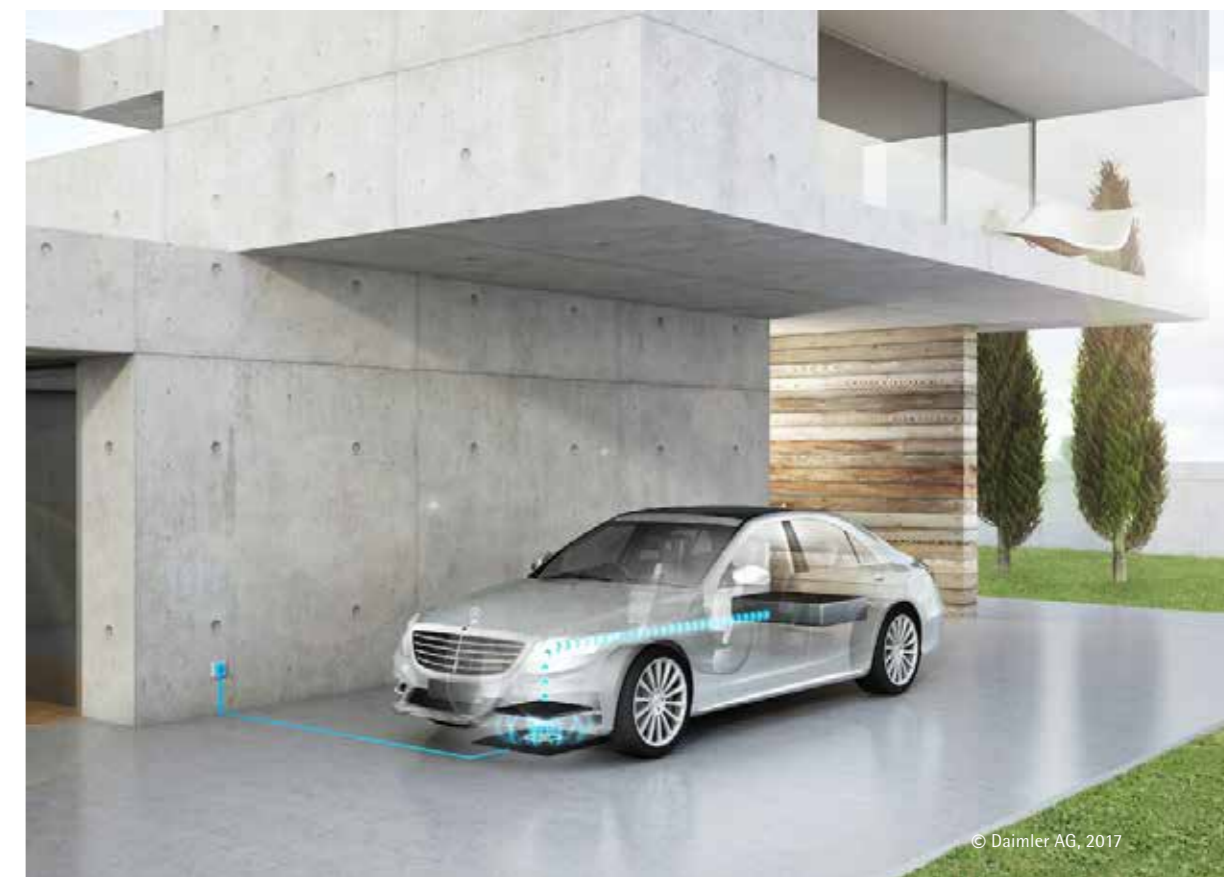
Cable-free charging through a secondary coil in the vehicle floor and a primary coil integrated into the baseplate
