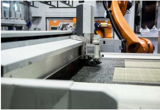
The fully automatic production process commences with an individually developed CF-SMC recyclate cutting system
