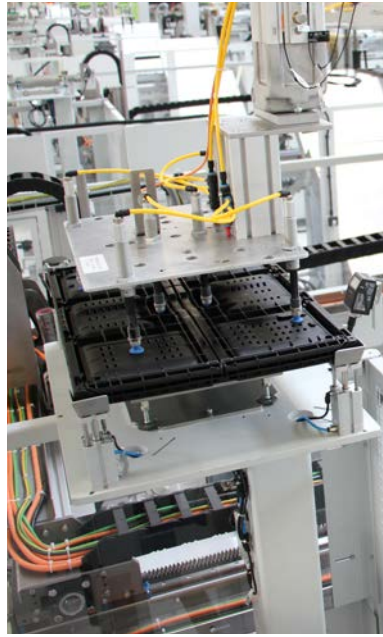
After injection moulding, a robot removes the various parts of the returnable box prior to their fully automatic assembly, labelling with an individual code and printing.
