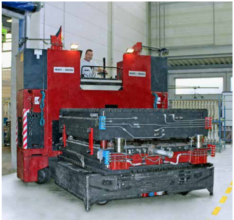
Optimization focused on the setting up of a 28t tool for the production of truck bumpers.
