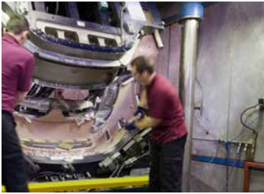
Bumper production using the PUR-RRIM process.
