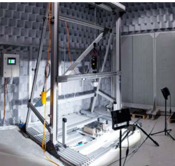
The data generated in a simulation is substantiated with a practical test on a drop tower.
