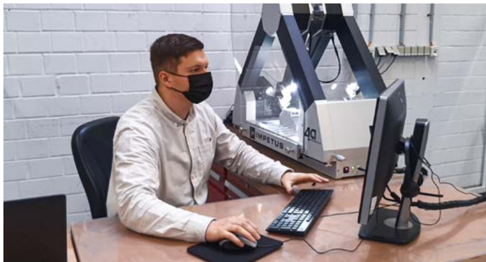
In 2021, POLYTEC invested in a test stand which can examine the strength of materials upon a high-speed pendulum impact.
