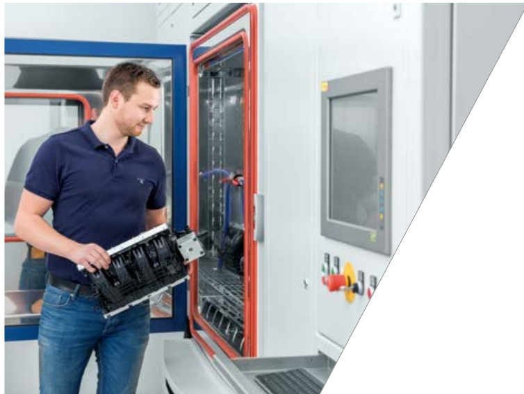
The pulsation test unit is used to scrutinise components for structural weak points.
