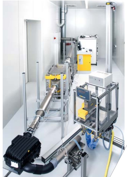
Examination of an air filter system on a test stand.
