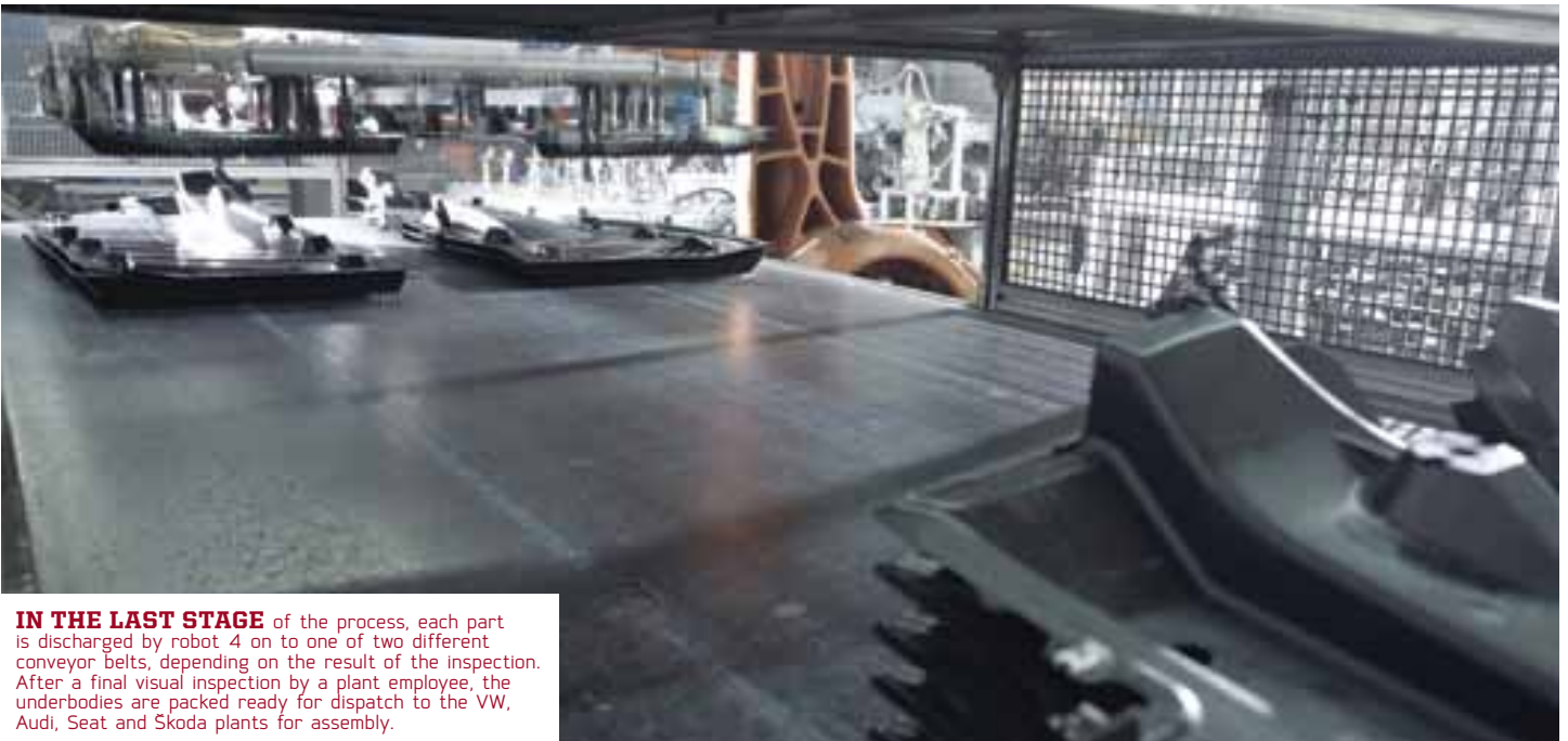
FULLY AUTOMATED STAMPING PROCESS: After the molded parts have cooled, they require no further processing. A conveyor belt carries the waste from the stamping process to a shredder, so that it can be mixed directly into the closed-loop recycling system and re-used for production of new parts. In a further step, robot 3 takes both components from the stamping tool and deposits them at the assembly station.
