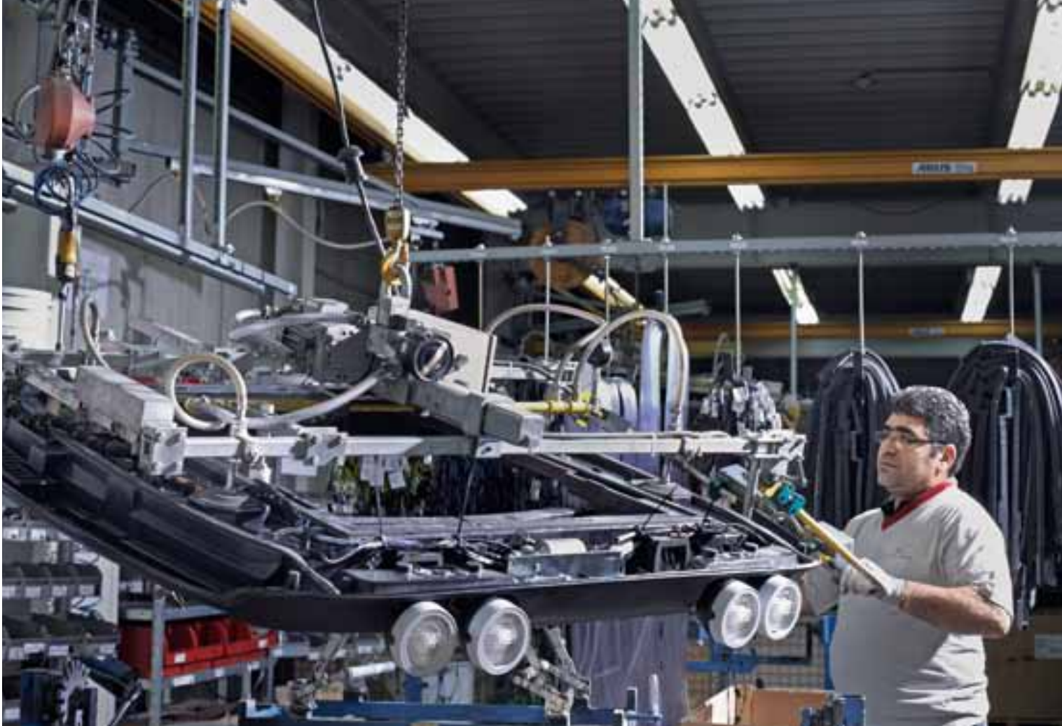
ASSEMBLY WORKER HACI B. assembling a John Deere tractor cabin roof at the Composites plant in Gochsheim.
