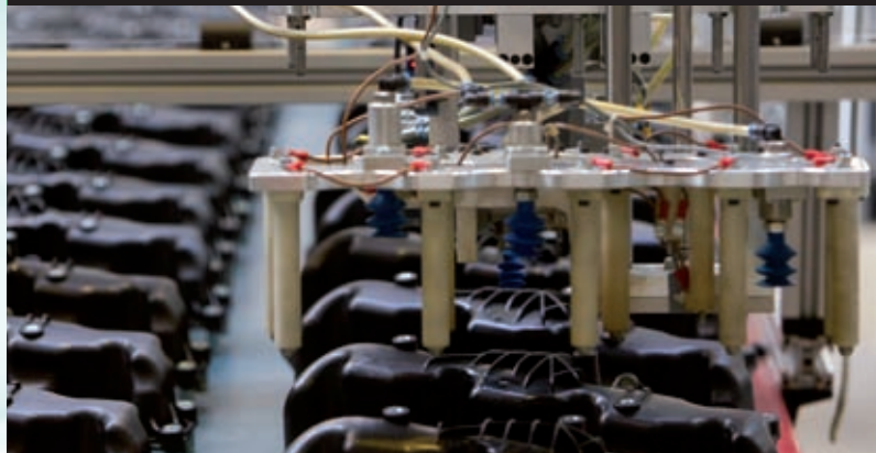
Product testing is a key priority – here the intake socket of the intake manifold.
