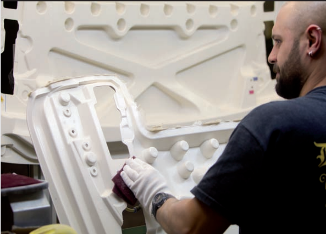
After milling, the sharp edges of all interior parts are removed manually.
