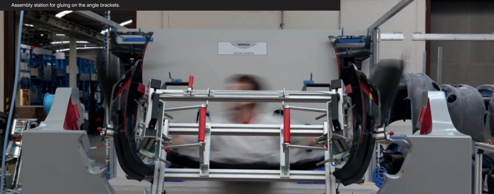
Assembly station for gluing on the angle brackets.
