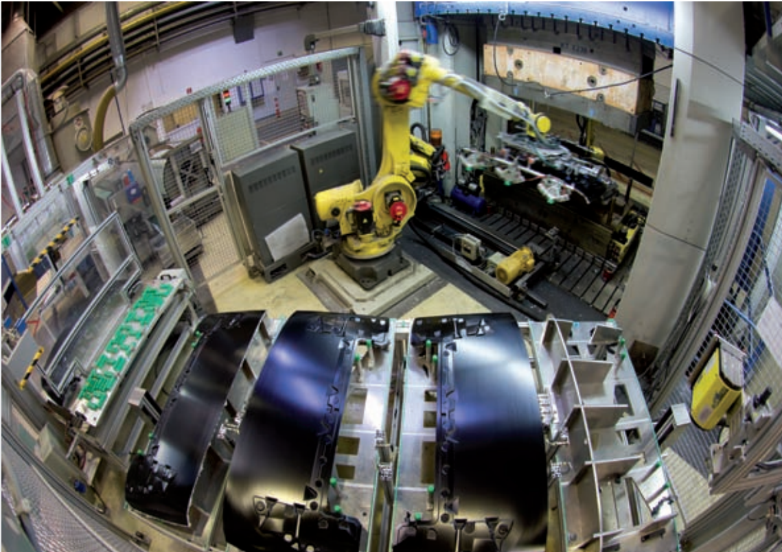
The loading of the tools with preformed SMC mats and the removal of the components is a fully automated process. After molding, the components have a temperature of around 140°C and are then cooled to below 50°C
